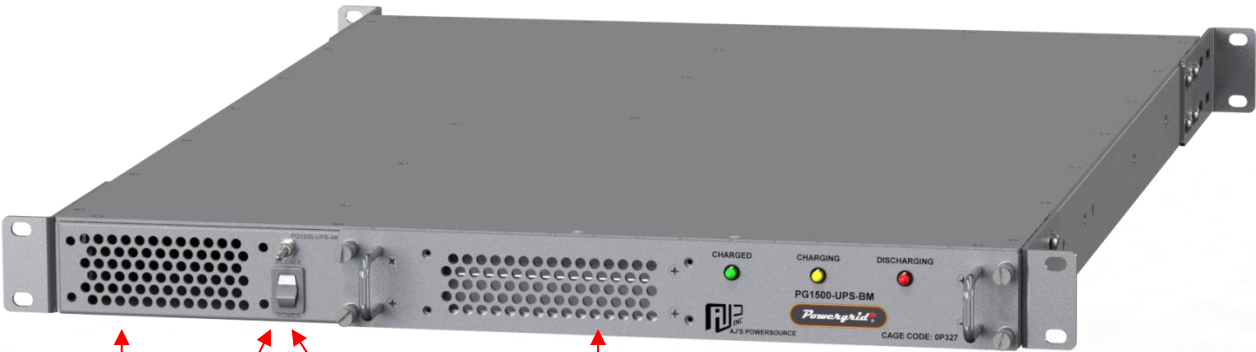
Air Intake Alarm Disable Output Enable Air Intake Battery Module
